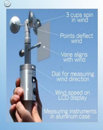
AN ANEMOMETER MEASURES WIND SPEED AND WIND PRESSURE.
