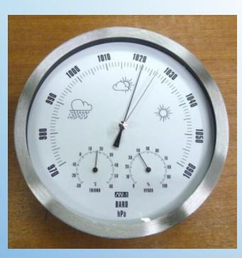
A BAROMETER MEASURES AIR PRESSURE.
