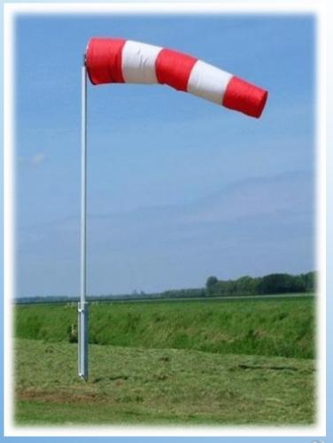
A WIND SOCK IS A CONICAL TEXTILE TUBE, WHICH RESEMBLES A GIANT SOCK, DESIGNED TO INDICATE WIND DIRECTION AND RELATIVE WIND SPEED.
